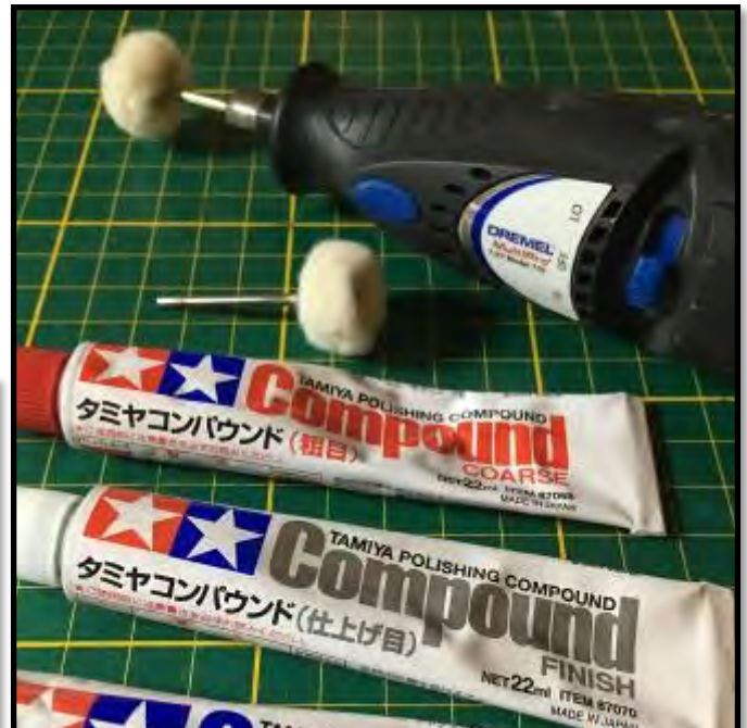
Removing cracks: Sand to 12000 first, then polish with Tamiya polishing compounds using a jewelers buffing wheel on a dremel, low speed. I dunk in future only if still necessary.
